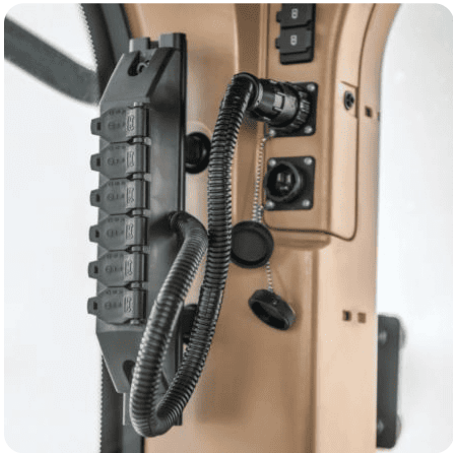
Convenience Power and Power Strip Outlets
