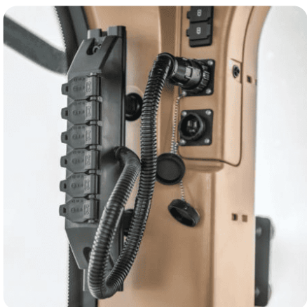
Convenience Power and Power Strip Outlets
