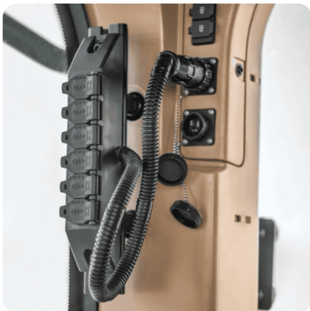
Convenience Power and Power Strip Outlets
